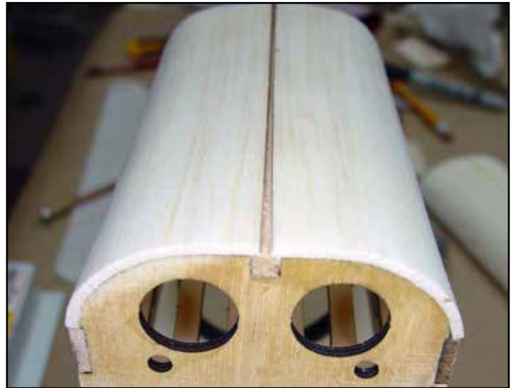
Sand the sheeting flush with former B and the fuselage sides.
