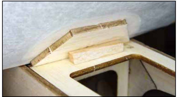
F15 is placed snugly against the wing and belly pan and glued to the fuselage. A piece of scrap 3/16" square is used to insure it retains that exact angle for a match to the belly pan.
