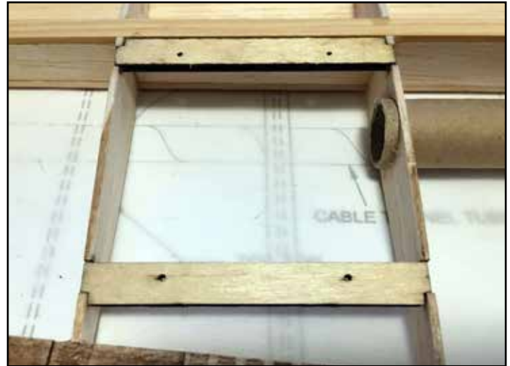
Install the servo rails and use some 1/4" length pieces of 1/4" triangle stock as gussets between the ribs and the rails.
