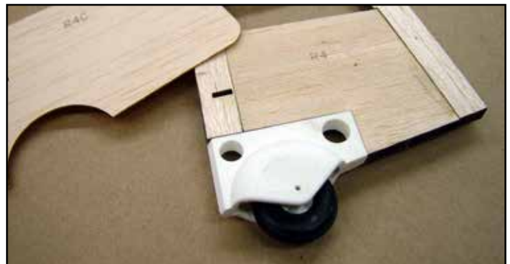
The assembled tail wheel is glued to the rudder with thick CA.
