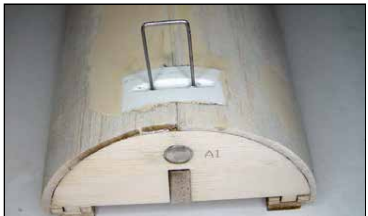
The hatch pull in the extended position. It will retract into the recess when not in use. You can access it with a fingernail or a magnet.
