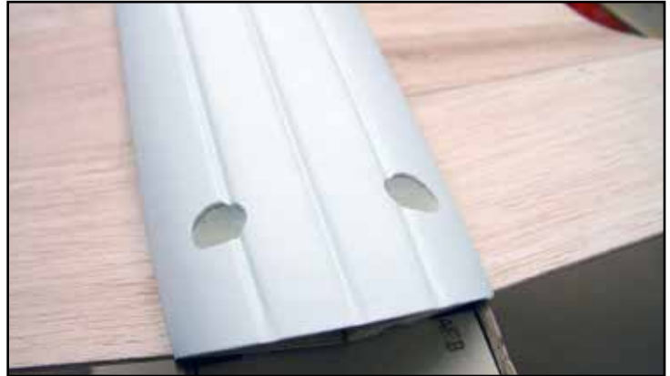
The marks transferred from the paper taped to the fuselage are carefully opened up to the diameter of the bolt wells.
