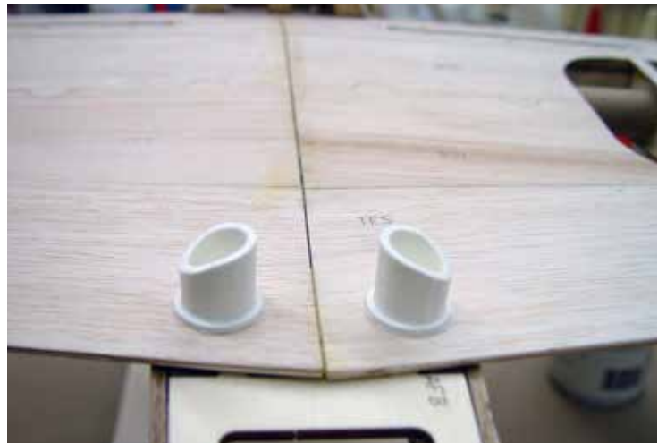
The wing secured to the fuselage with the wing bolt and the two bolt wells.
