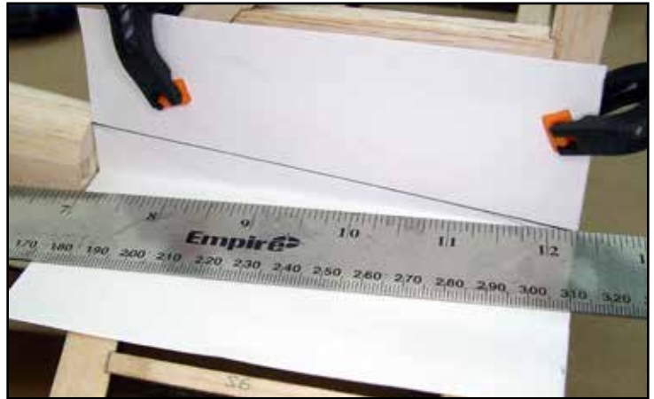
A paper template is made to mark the angles on the tail block. The top angle has been marked and then the clamps were moved from the stabilizer to the fin and now the side angle is being marked.
