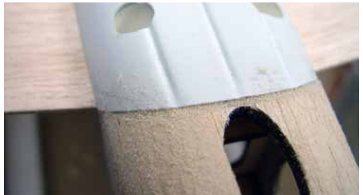
The aft fuselage bottom has been shaped to contour with the belly pan.
