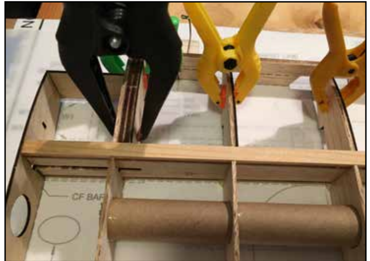
Steps 19, 20 and 21, laminating the gear block assembly as well as W3-A and W4-A, clamps are used to insure good contact with the paring ribs.
