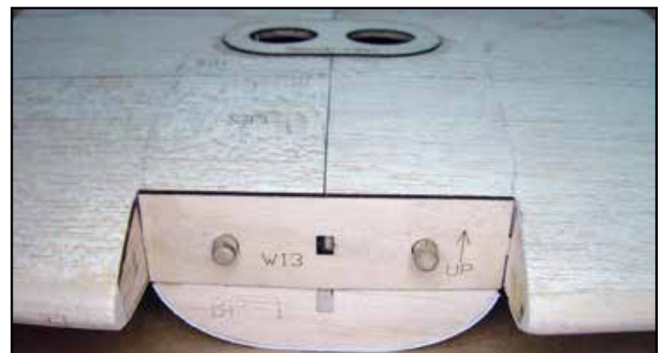
Completed wing assembly, the correct dihedral is set by W13. Note the Cable opening plate. NOTE: In this photo the belly pan has been installed. You will install that later in the build.
