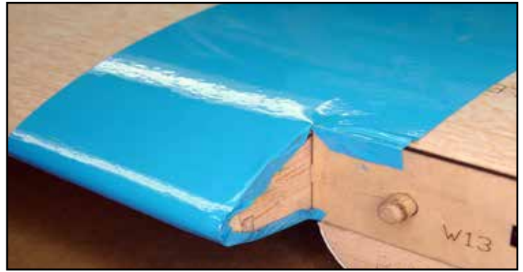
A temporary strip of MonoKote is applied to the wing in the area of the fuselage. Be sure to wrap it over the edges as shown here.
