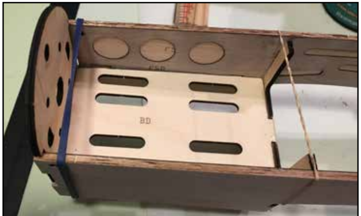
Use Epoxy to install the battery deck assembly
