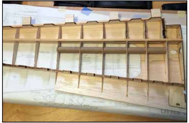
Except for the area along the spar, the top leading edge sheeting is glued from the open bottom with thin CA.
