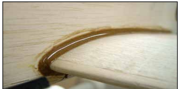
After removing the temporary MonoKote the fillet will give it a great finished look to your model.
