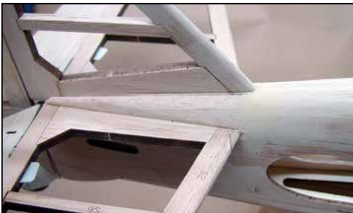
Much of the rounding over and shaping can be done before the blocks are glued in place.
