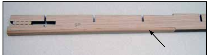
SD-BOT has been installed onto the spar, next the 3/32" x 1/4" spruce will be added.
