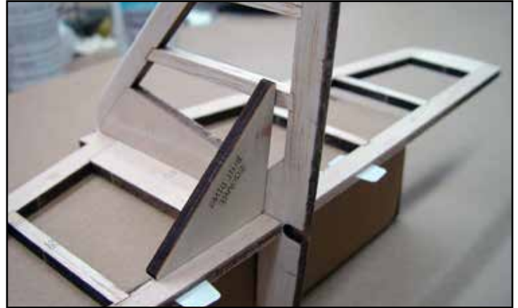
The stabilizer is raised by placing it on a box and the vertical fin is installed and glued at 90° to the stabilizer.
