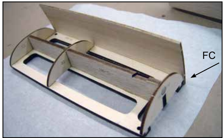
The whetted hatch sheeting is first glued to HA-A and then rolled over onto the formers and HA-HA-C and glued with thin CA.
