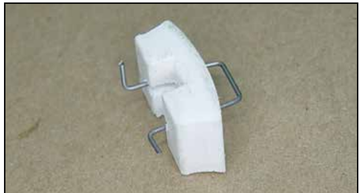
The hatch pull assembly ready to be installed into the hatch. The pull wire will retract into the hatch when not in use.
