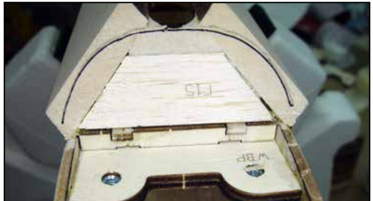
The wing is attached and the belly pan is used to draw the matching contour onto the aft fuselage parts after they have been sanded flat to F15.
