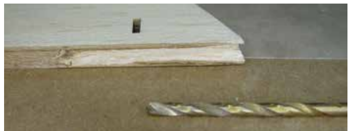
Dragging a drill bit on it's side makes a great tool for digging the groove in the leading edge.
