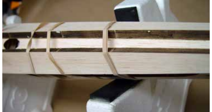
Two F17 corner pieces are held in contact with the fuselage sides and F16 with rubber bands.
