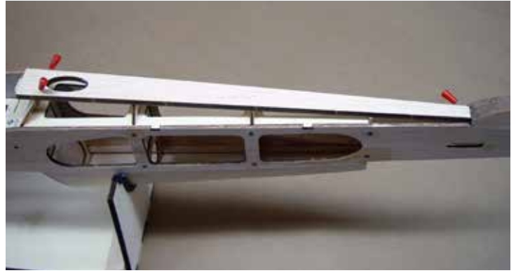
F16 has been glued to the bottom formers and the tail skid block.
