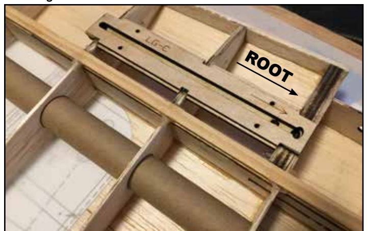
When the gear block is installed, LG-C should stand 1/16" proud of the ribs. This will bring it flush with the top of the leading edge sheeting when installed.
