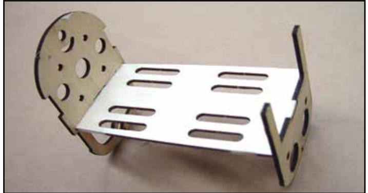
Former A (firewall) and former B assembled with the battery deck (BD). Use the square to keep all these components square to each other.
