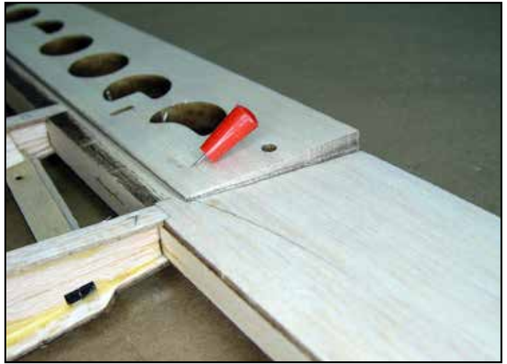
Marking the aileron for shaping to the contour of the wing. Mark the leading edge top and bottom as well as both ends. The tip can be marked by laying a straight edge on the tip and projecting a line over the end of the aileron.
