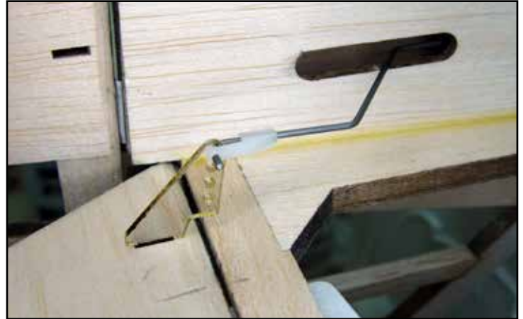
The elevator horn and linkage is temporarily installed before the model is covered. Note that the fuselage exit guide will also be installed after the model is covered.
