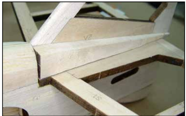
Much of the rounding over and shaping can be done before the blocks are glued in place.
