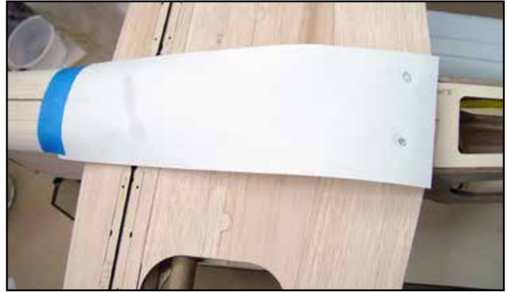
A piece of paper temporarily taped to the fuselage with the bolt holes marked on will transfer the location of the bolt holes to the belly pan.
