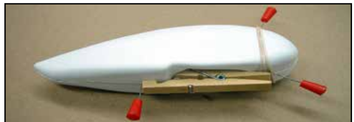
Glue the outboard half of the wheel well shell to the inboard assembly.
