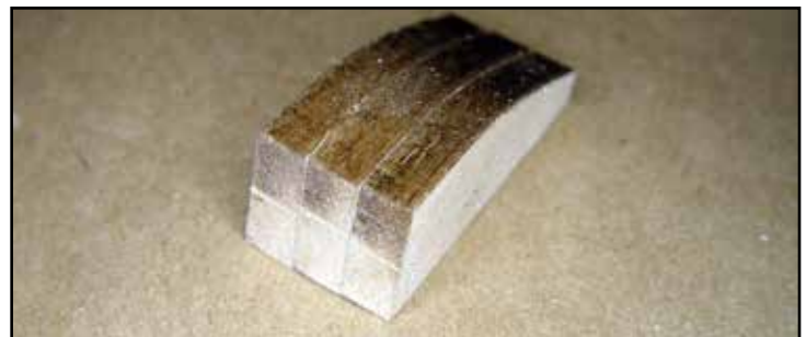
The tail skid laminated from three SF parts.
