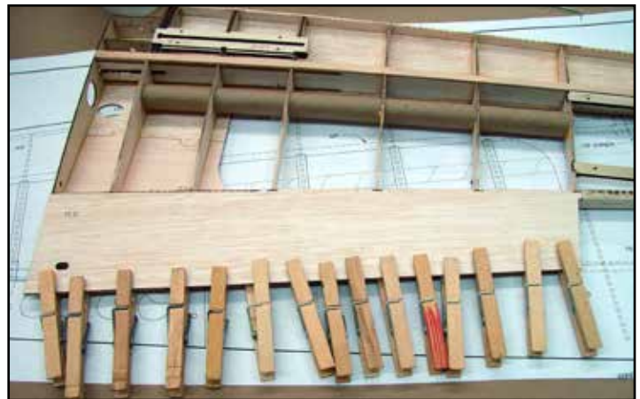
When installing the bottom trailing edge, use plenty of clamps along the trailing edge. A slight taper on both sheets will yield a nice crisp trailing edge.
